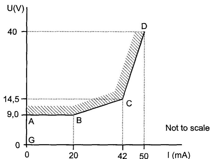
Figure 3 - TE voltage/current characteristics
