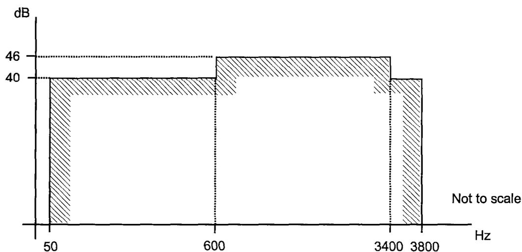
Figure 6 – Output Signal Balance and Longitudinal Conversion Loss, minimum values
