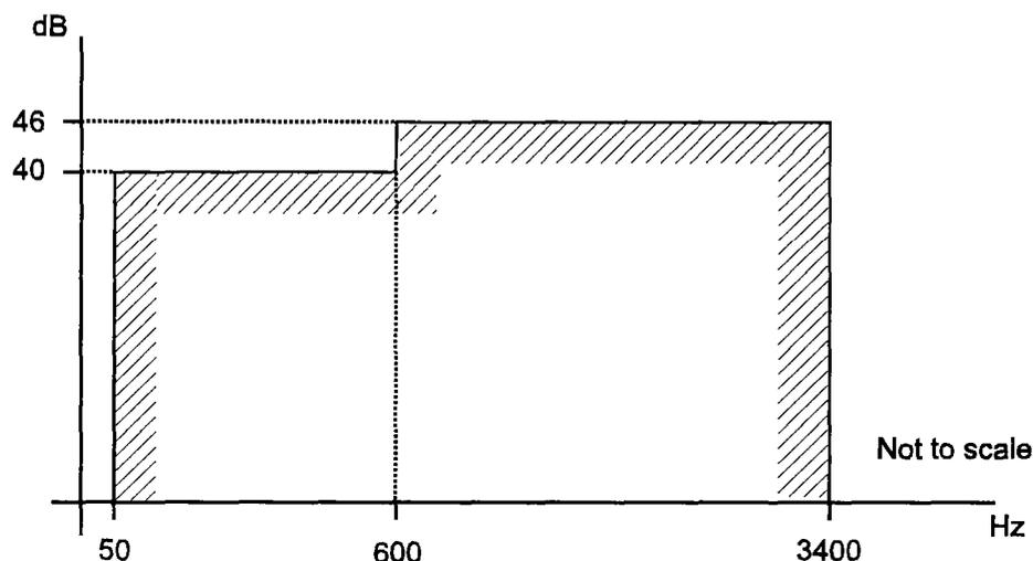
Figure 2 – Longitudinal Conversion Loss, minimum values
