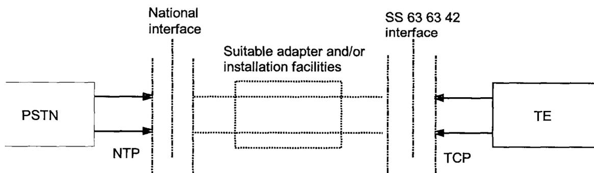
Figure 1 – Network Termination Point (NTP) and Terminal Connection Point (TCP)
