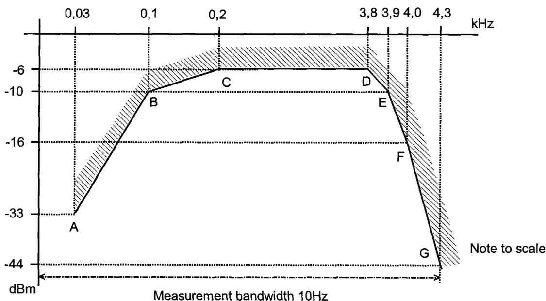
Figure 4 – Power level in a 10 Hz bandwidth
