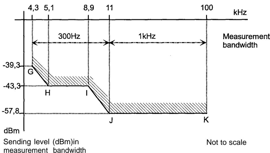
Figure 5 – Sending power level above 4,3 kHz
